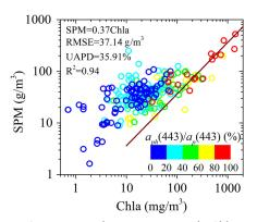
**Fig. 14.** Comparisons between measured Chla and SPM. Relationship between SPM<sub>*ph*</sub> and Chla (solid line) was derived using data with  $a_{ph}(443)/a_p(443) > 80\%$  (red circles).
