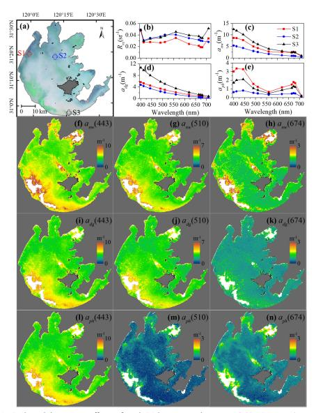
**Fig. 12.** Example of OLCI-derived absorption coefficients for Lake Taihu on December 08, 2016: (a) RGB image (R, Band 10; G, Band 6; and B, Band 3); (b)–(e) OLCI-derived  $R_{rs}(\lambda)$ ,  $a_{nw}(\lambda)$ ,  $a_{dg}(\lambda)$ ,  $a_{ph}(\lambda)$  from three sites (S1–S3), representing different bio-optical properties. Spatial distributions of (f)–(h)  $a_{nw}(\lambda)$ , (i-k)  $a_{ph}(\lambda)$ , and (i)–(n)  $a_{dg}(\lambda)$  at 443, 510, and 674 nm, respectively.
