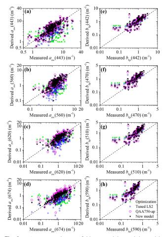
**Fig. 8.** Comparisons between field-measured data and the models (the nonlinear optimization method, tuned LS2 model, QAA750-ap, and the proposed new model) deriving  $a_{nw}(\lambda)$  at 443, 560, 620, and 674 nm and  $b_{bp}(\lambda)$  at 442, 470, 510, and 590 nm [four bands of the *in situ*  $b_{bp}(\lambda)$ ].
