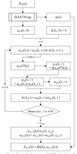
**Fig. 2.** Flow chart of the proposed IOP algorithm for fieldmeasured data. Remote sensing reflectance  $[R_{rs}(\lambda)]$  is the input parameter obtained from field measurements.  $u(\lambda) = b_b(\lambda)/(a(\lambda) + b_b(\lambda))$ . Details of QAA750-ap are described in Table 1.
