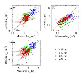
**Fig. 10.** Comparisons between measured and model-derived (a)  $a_{nw}(\lambda)$ , (b)  $a_{ph}(\lambda)$ , and (c)  $a_{dg}(\lambda)$  at 443, 560, 620, and 674 nm (N = 57). Note that the error bars of the measured  $a_{nw}(\lambda)$  and the measured  $a_{dg}(\lambda)$  are based on the uncertainties in the estimated  $a_p(750)$ .
