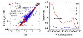
**Fig. 5.** (a) Comparisons between field-measured  $a_{pb}675$  and LH derived from field-measured  $a_{nw}(\lambda)$  and  $a_{nw}(\lambda, i = 0)$ , respectively. The black line is the equation fitted from field-measured  $a_{nw}(\lambda)$ . (b) Parameters  $(B_0, B_1)$  and  $R^2$  of the relationship between the field-measured  $a_{pb}(\lambda)$  and  $a_{pb}675$  in Eq. (14).
