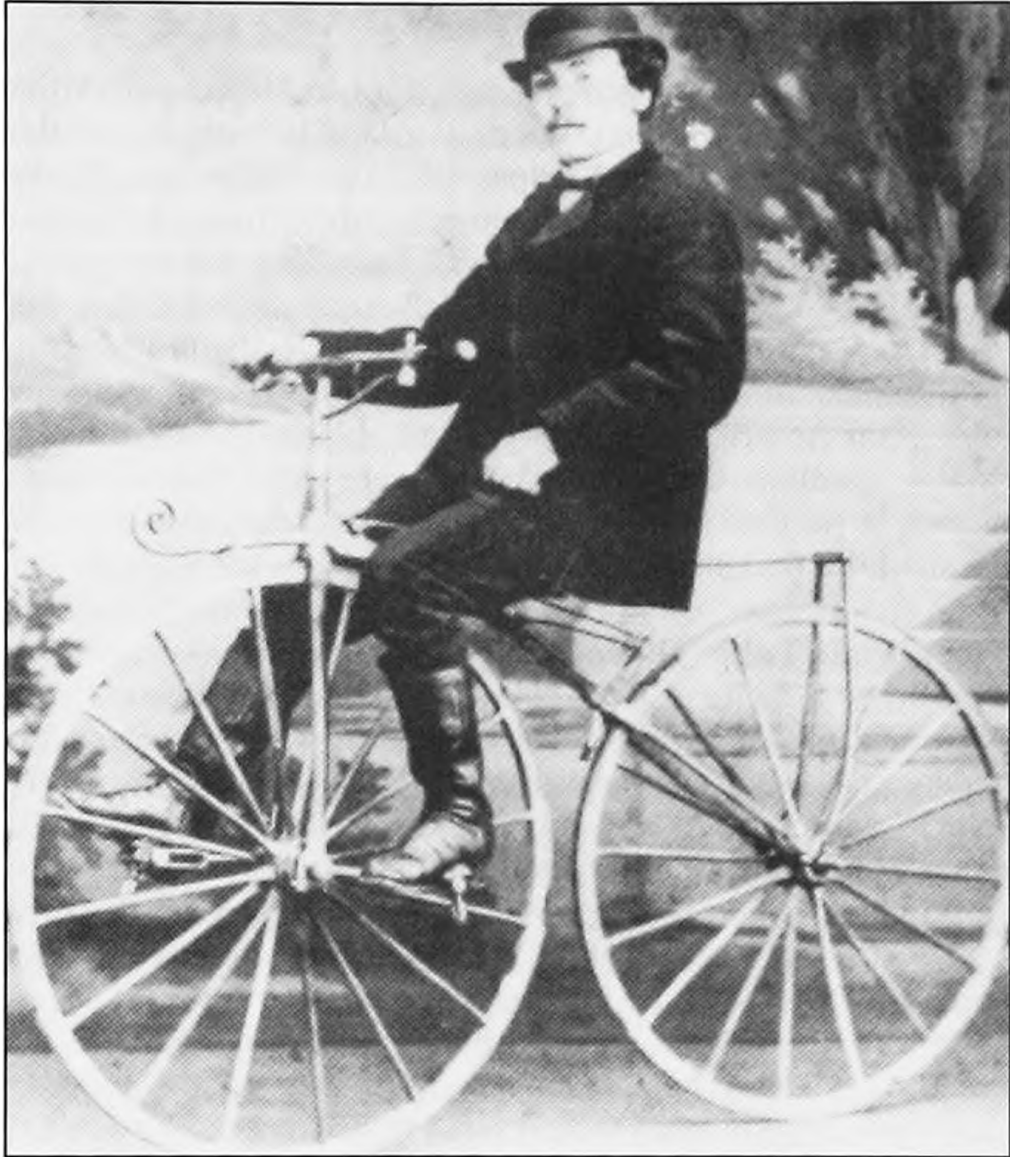
Pierre Lallement, a young mechanic, introduced his new velocipede in Paris in 1863. Although crude by modern standards, these first bicycles were considered speedy, compact, and dashing, and they opened a door to developing a practical means of personal transportation. The new vehicle found fertile ground in Maine in 1868-1869, with Portland boasting one of the nation's first and largest velocipede manufacturers. Photo from THE CYCLE [BOSTON, JULY 2, 1886], courtesy Lallement Memorial Fund Drive and the author.
