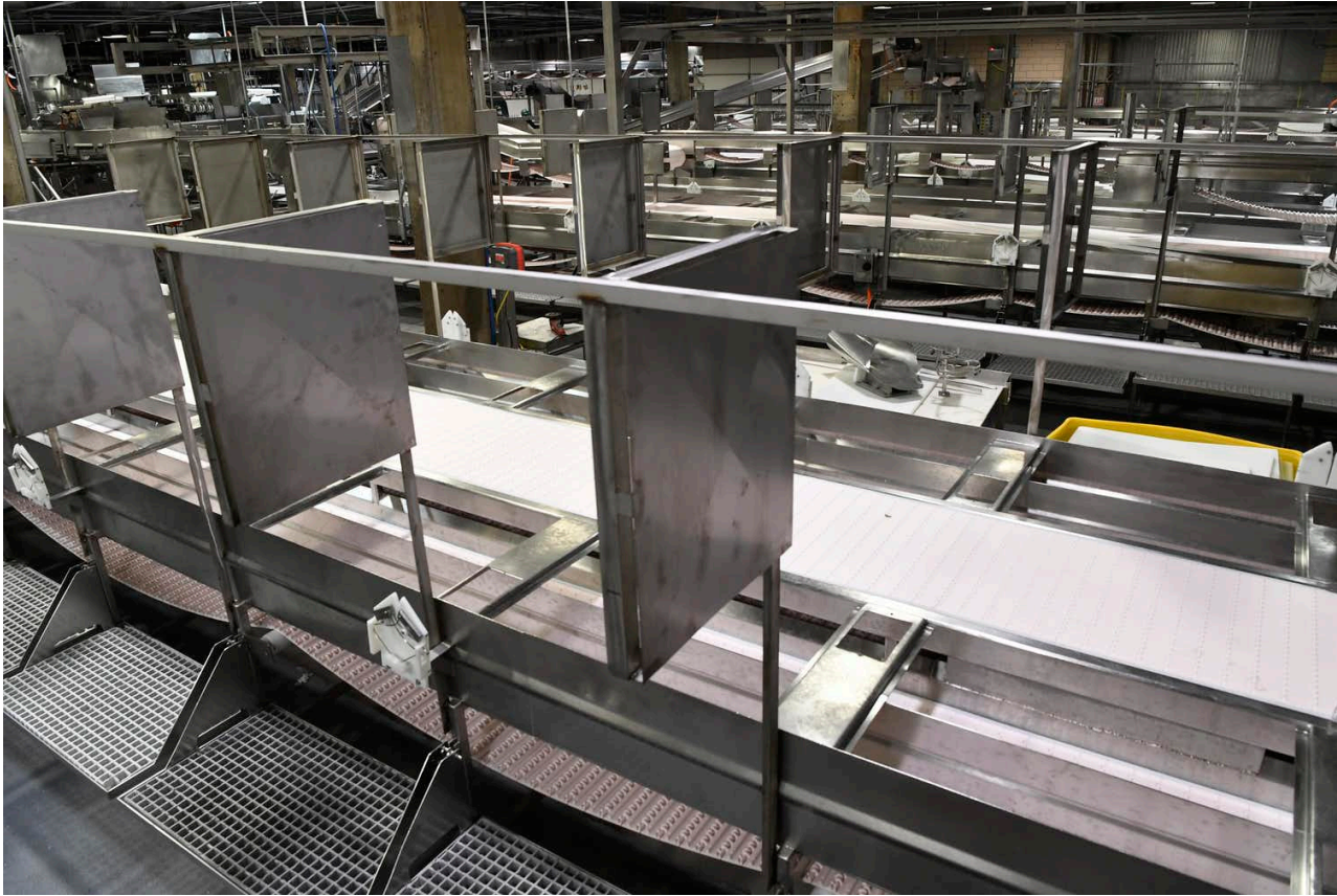
Meat processing stations at the JBS Beef Plant in Greeley, Colo., equipped with new sheet-metal partitions, April 23, 2020. As of early May 2020 the plant had recorded more than 200 confirmed cases of COVID-19 and 6 employee deaths. Andy Cross via Getty Images
