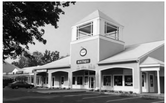
Long commercial buildings should have a focal point and/or an offset in the roofline to break up their mass.
