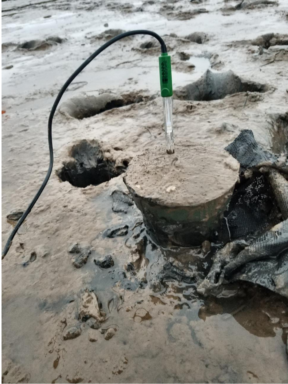
Measuring pH in an EU with the protective netting removed
