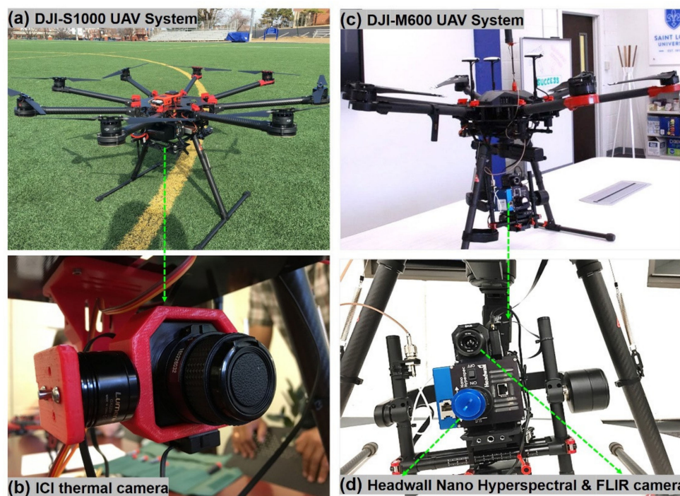
Figure 2. UAV systems and interrelated sensors. DJI S1000+ UAV system (a) with ICI thermal camera (b), DJI-Matrice 600 Pro UAV system, (c) with Headwall Nano Hyperspectral and FLIR thermal cameras (d).
