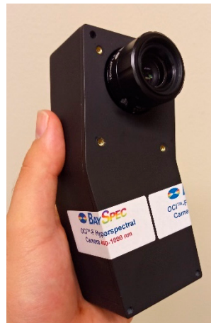
Figure 3. Shows the BaySpec hyperspectral camera used for recording these values. The range of the camera is from 400 to 1000 nm.
