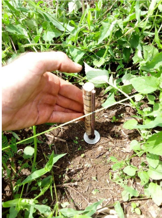
Figure 8: An erosion pin installed using a 15 cm wooden peg (shown with black rings around it), a washer, guide rope, and wooden mallet (not shown). (Photograph taken by author)
