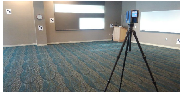
Figure 2. Test field scanning by FARO Scanner
