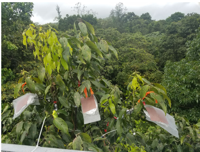
FIGURE 4 Examples of leaf heaters in the upper canopy of Ocotea sintensis , part of the Tropical Responses to Altered Climate Experiment (TRACE) in the Luquillo Experimental Forest in Puerto Rico (photo credit M. Cavaleri) [Color figure can be viewed at wileyonlinelibrary.com ]
