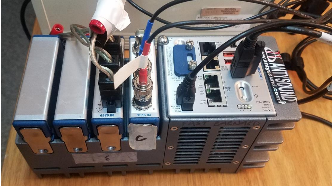
Figure 108: cRIO 9031 Configured to Serve as an ANC Controller
