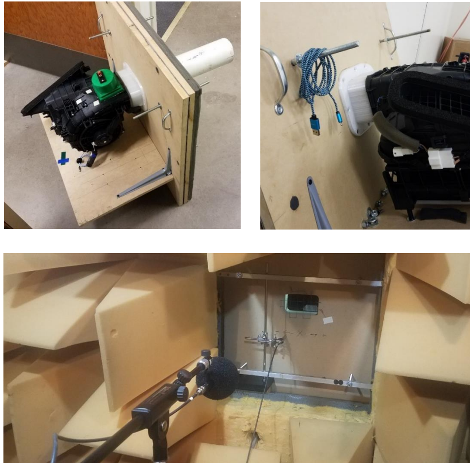
Figure 7: Installation of Blower Fan onto Partition: Fan Outlet in Anechoic Chamber
