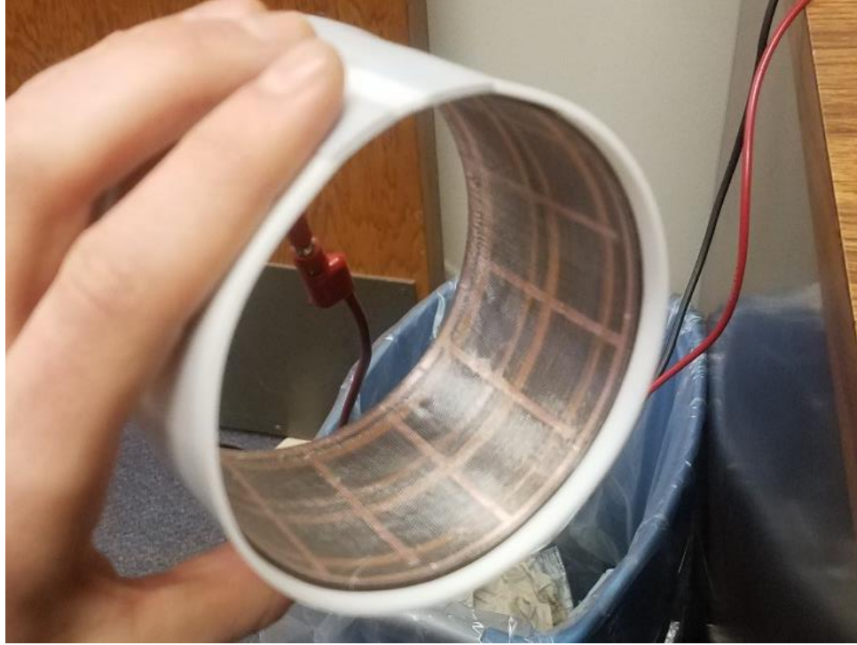
Figure 104: Close up of Annular Teflon Speaker Construction
