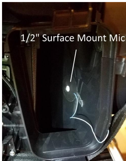
Figure 34: Detail Placement of Surface-Mount Microphone Location Used for Characterization of Sources Inside the Blower Fan in the Full HVAC Configuration
