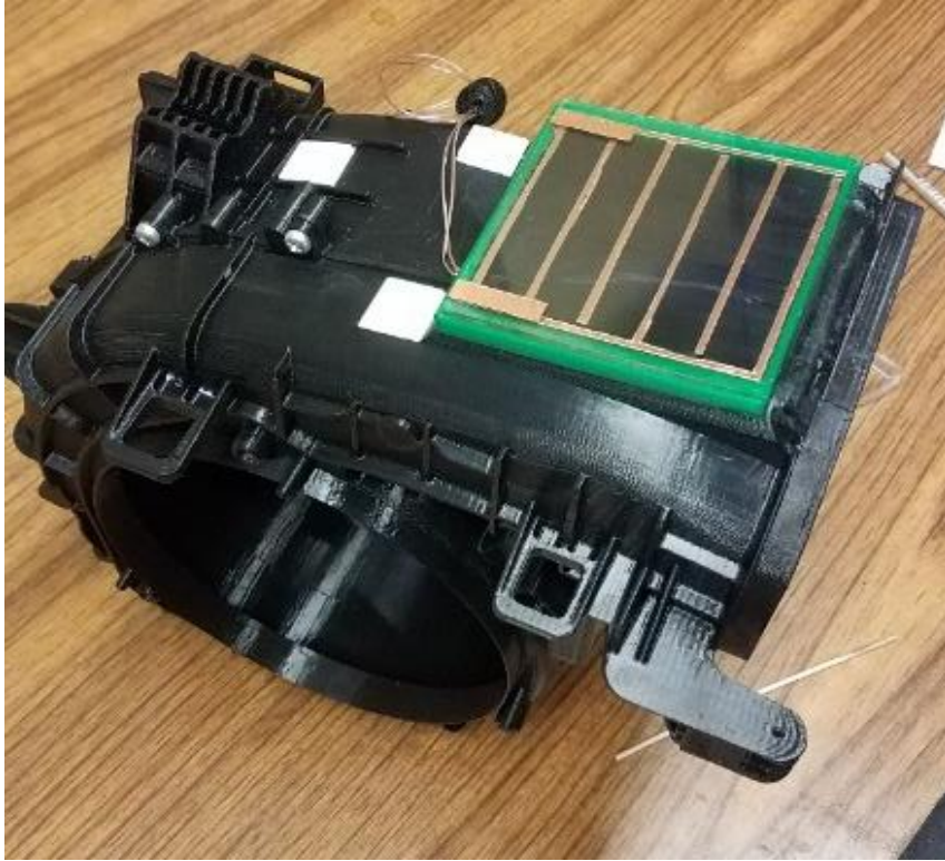
Figure 101: Glass Rigid CNT Panel Installed onto RC03 Prototype Thermophone Using a 3D-Printed Adapter
