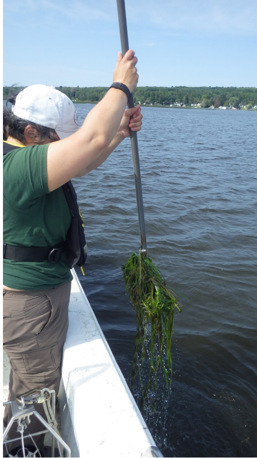
Figure 3.7. Rake twist sample immediately after retrieval from the water from an area with dense SAV, undergoing visual estimation of density.
