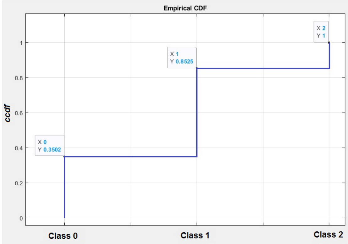
Figure 5. Cumulative conditional distribution function ( ccdf ) plot for selecting random pattern by drawing a random sample from the probability distribution for highly crowded clusters.
