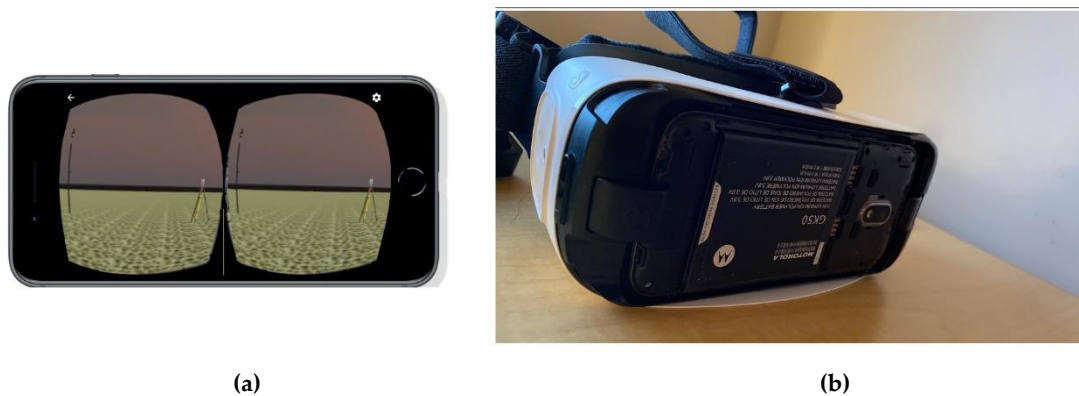
Figure 6. (a): a demo of an implemented VR application on an Android smartphone. (b): a view of the smartphone inside the Samsung VR goggles.
