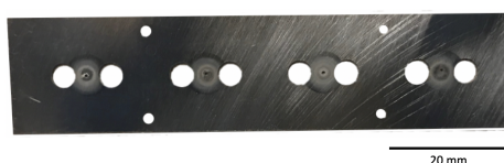
Figure 2. A photograph of the side of the anode facing the cathode components. During testing, the small pinholes at the center of each discolored ring are directly in line with the cathodes.
