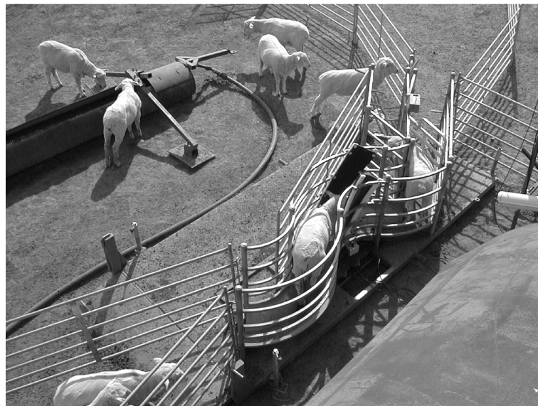
Figure1 Remote weighing and automatic drafting facility showing the curved race which encourages animals to pass slowly over the weighing platform while entering a watering enclosure , tag reader ( located in the race ) and drafting gates .
