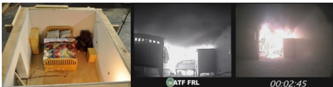
Fig. 25. Scale modeling of a bedroom fire.
