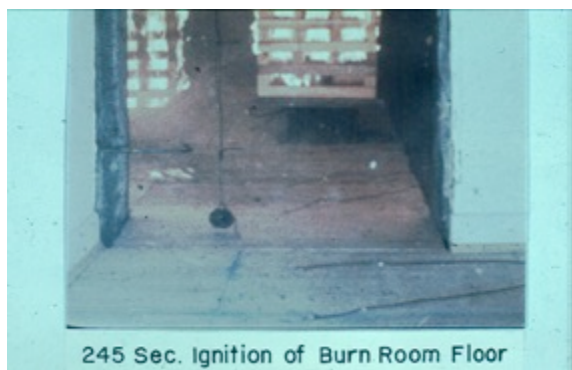
Fig. 1. Fire spread into a corridor on a wood floor.
