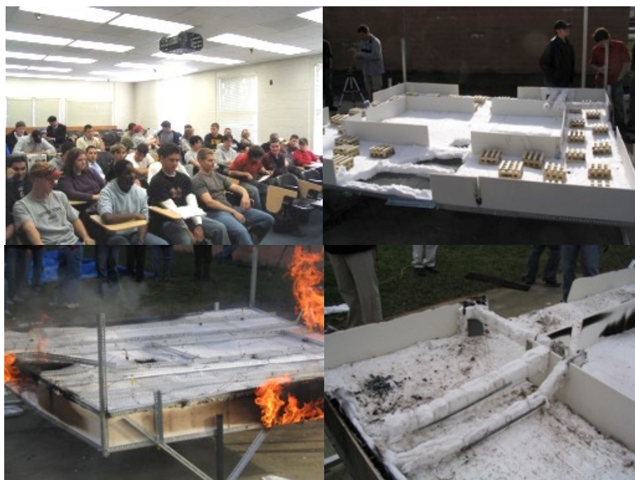
Fig. 23. Aspects of scaling a floor of the North WTC Tower fire.
