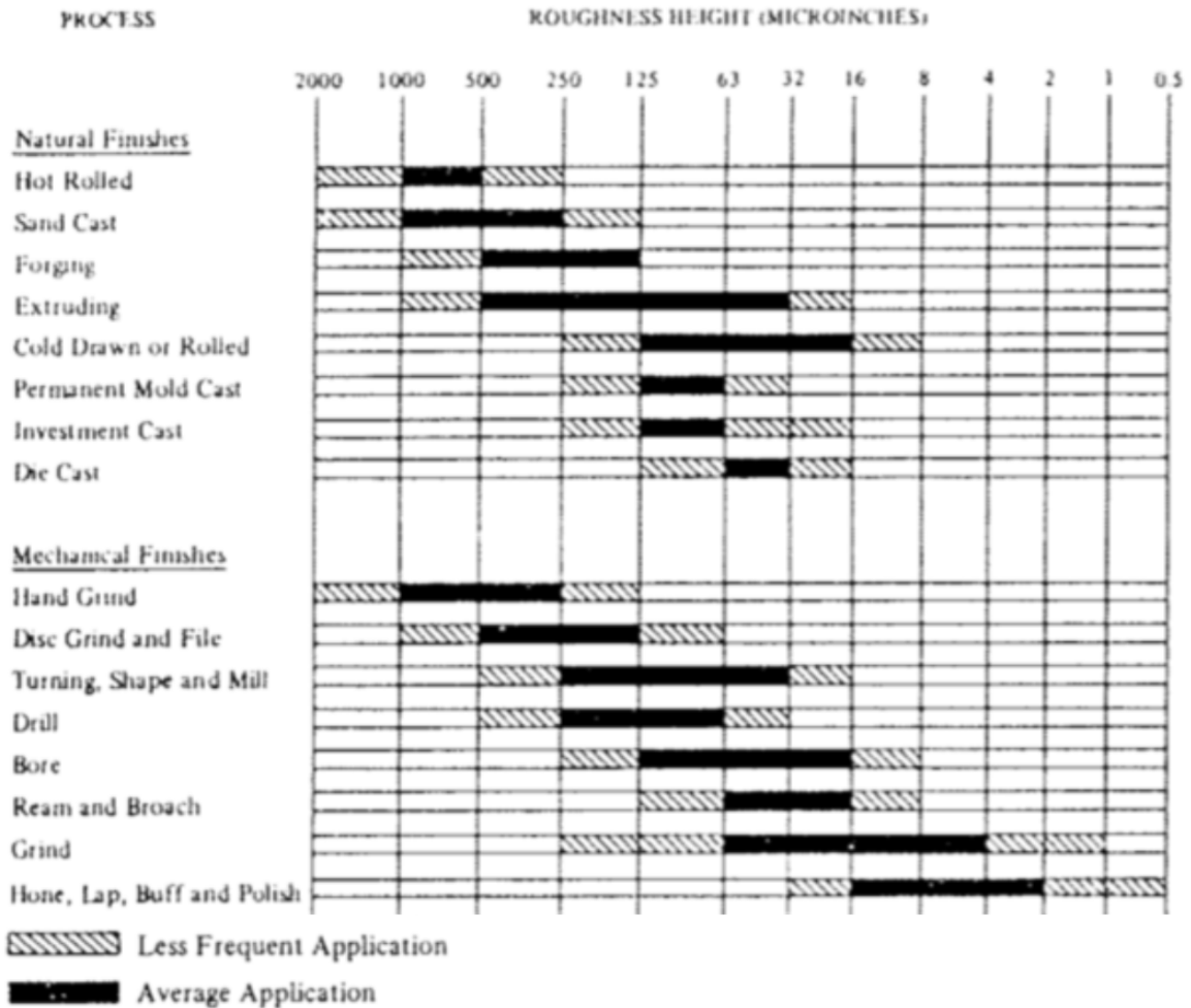
Figure 2.1. Surface roughness produced by common methods (modified from [2] with permission of Elsevier Inc., submission ID 1035201).
