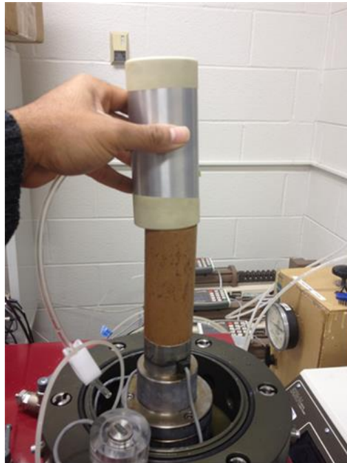
Figure E.11 Process of mounting an unsaturated specimen on the triaxial device
