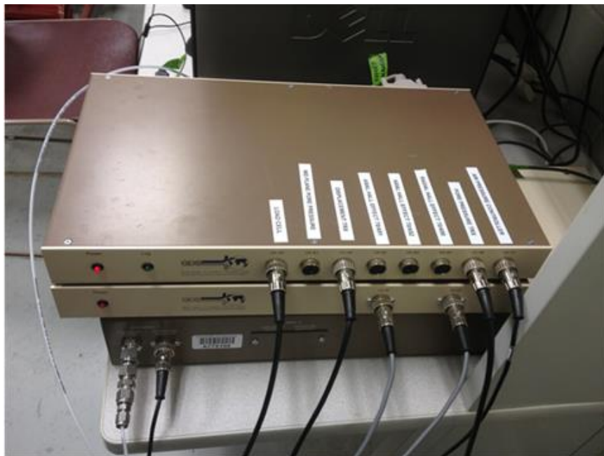
Figure E.7 Control boxes for coupled Bender Element-unsaturated triaxial testing: (top) data acquisition system, (middle) Bender Element control box; (bottom) GDS pneumatic pressure controller
