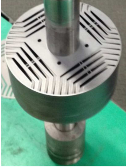
Fig. 16. Prototype rotor during manufacturing; the axial modular stagger skew further reduces the torque ripple from the 2D CE-FEA calculated values reported in other figures.
