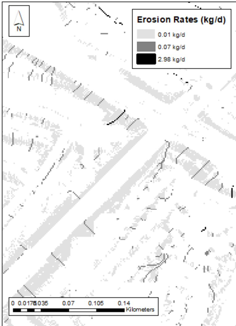
Figure 1.12. Connected areas and the erosion rates for connected cells for a road network on day 72 of 2006.
