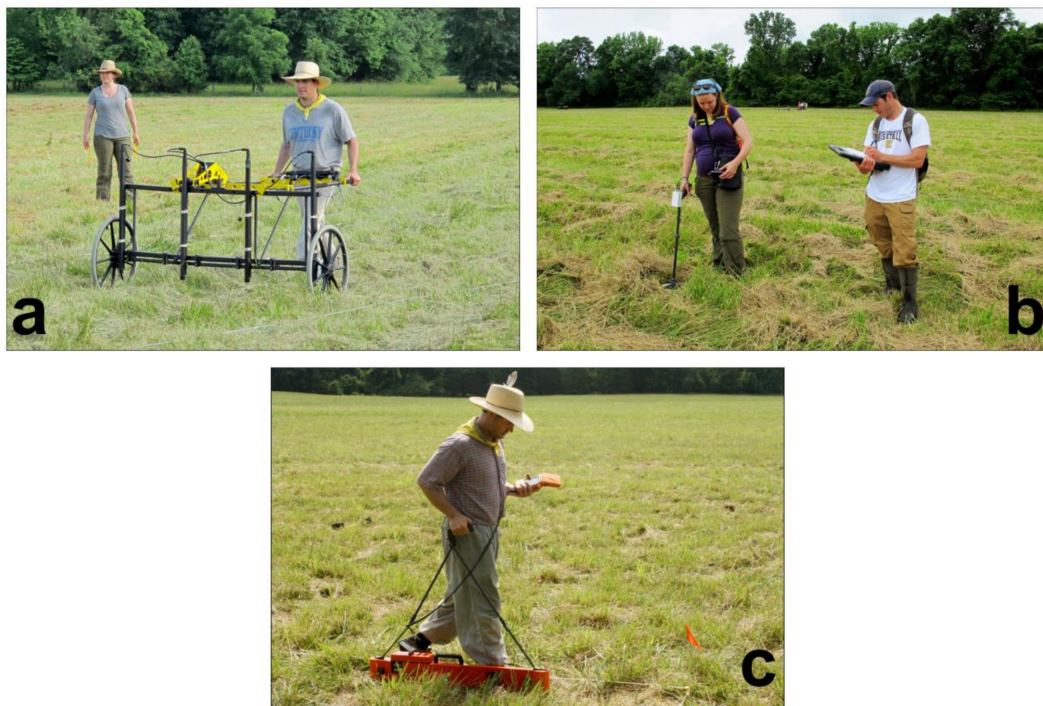
Figure 4. Geophysical data collection underway at the Johnston Site. (a) ERH collecting gradiometer data with the Foerster Ferex DLG Karto; (b) APW collecting magnetic susceptibility data using the Bartington MS2 m and the MS2D field loop; (c) ERH collecting EMI data with the Geonics, Ltd. EM38-MK2.
