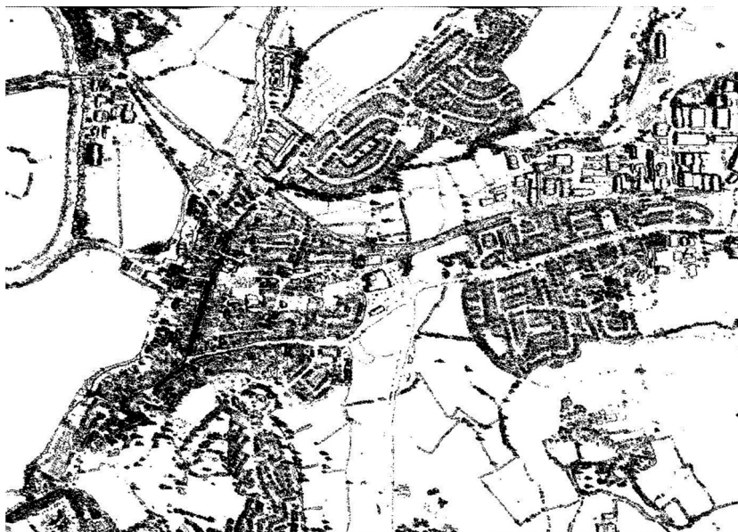
Fig. 3. Regions unseen (black) by TerraSAR-X in LiDAR DSM due to combined shadow and layover (satellite looking West) (after Mason et al., 2010).
