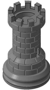
Figure 6: Chess Rook containing 93,930 triangles, dimensions: 31.75 x 31.75 x 53.15mm
