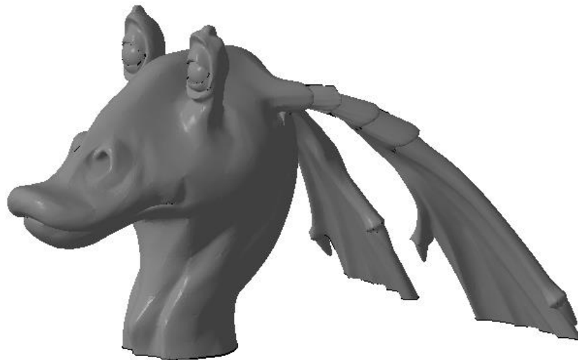
Figure 16: Figure head containing 467,882 triangles, dimensions of 141.61 x 111.27 x 81.29mm
