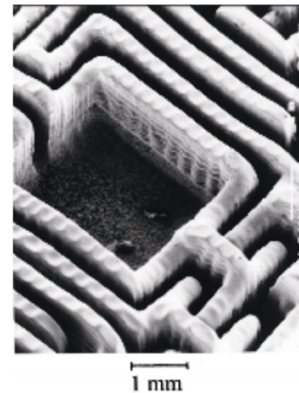
Fig. 16 SEM image of the sintered maze built by ink-jet printing. Reproduced with permission from Ref. [118], © The American Ceramic Society 2002.
