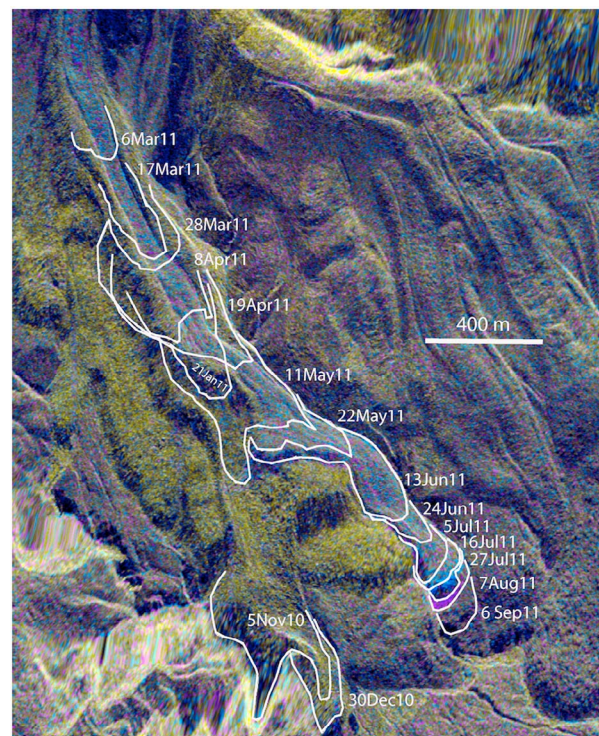
Figure 7. The mapped advance of the flow front positions on the dates shown, mainly for P2. The background change difference image is for 27 July–7 August 2011.
