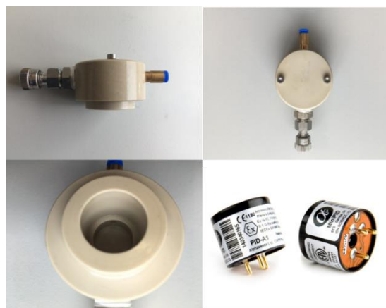
Figure 2.6. Detection Component. Different angles of the PTFE housing built for the PID (photoionisation detector, bottom right). The housing consisted of an input and output flow paths. The PID was mounted on a control board, which was then held in place with a clamp.
