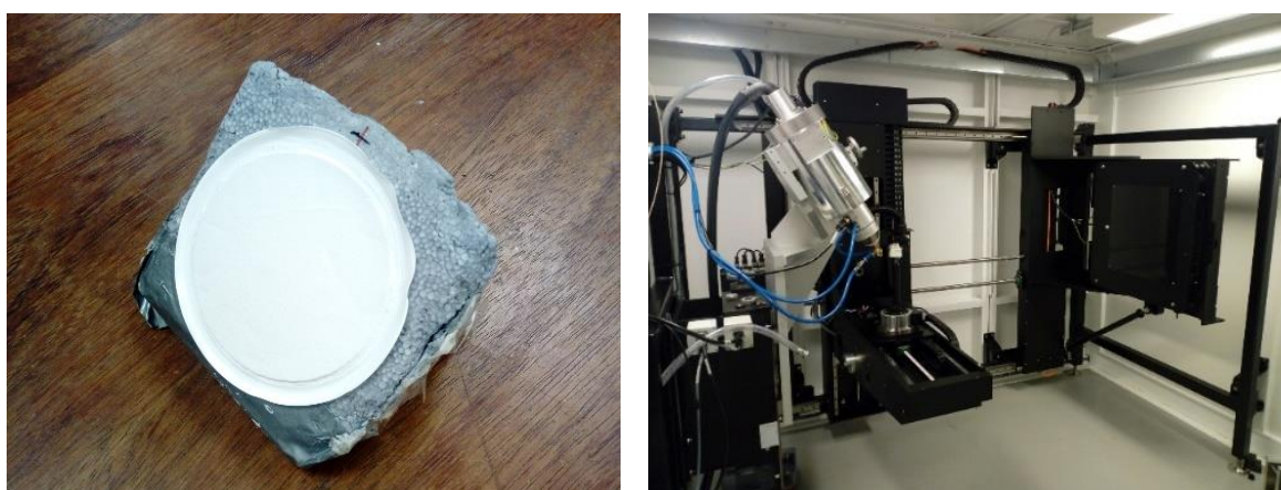
Figure 2.4: A cake sample placed on the sample holder used for imaging (left) and the High Flux Nikon XTEK bay at the University of Manchester used for XRCT imaging (right)
