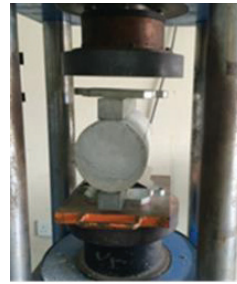
b) Splitting Tensile test
