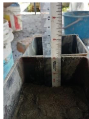
Fig. 7. 50 mm Gap at the Bottom of the Specimen
