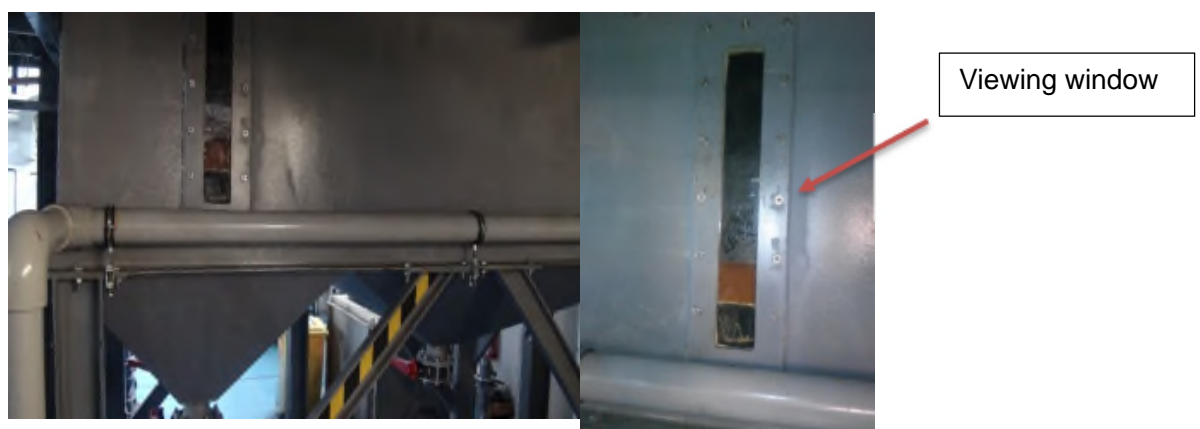
Figure 3-9: 3-Inch test facility separator with its viewing window
