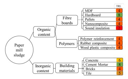
Fig. 2. Material applications from paper mill sludge
