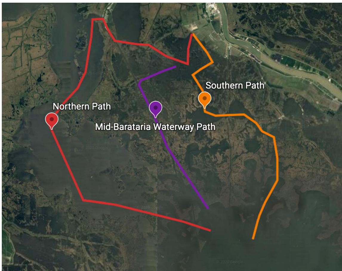
Figure 4.3: Three major distributary channels established by the Mid-Barataria Sediment Diversion.
