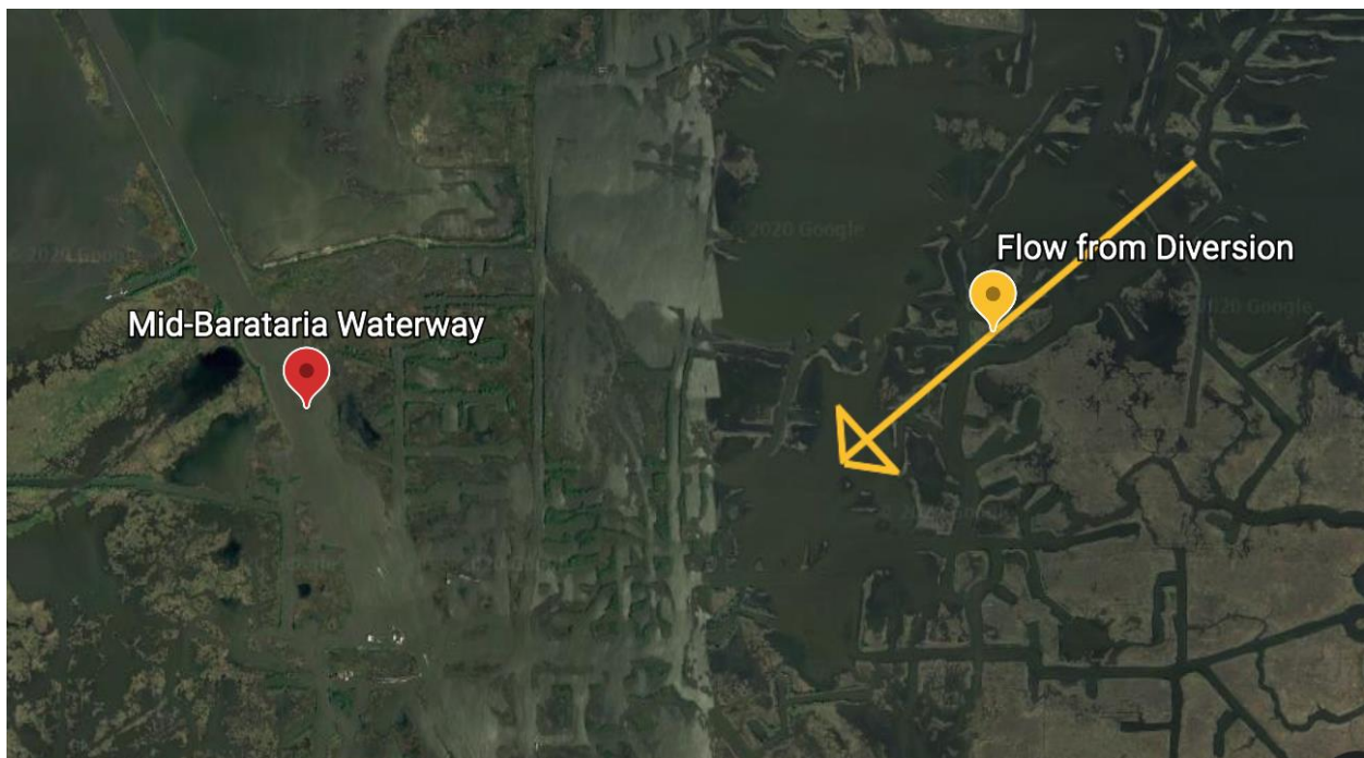
Figure 5.5: Open water distributaries that when combined increase the flow in the Barataria Waterway flowing south to create the Mid-Barataria Waterway diversion distributary channel. Observation points in red and flow paths in yellow.
