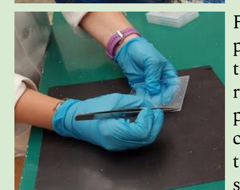
Fig 13: The protective film on the tiles need to be removed, and excess paint has to be chipped off, before the tiles can be shipped.
