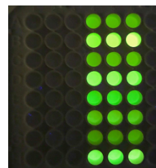
Figure 10: Well plate showing results from a fluorescence assay. High fluorescence represents high Hcy concentration and low enzyme activity.
