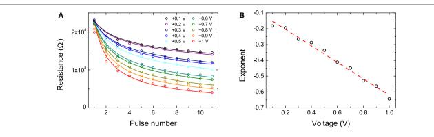
**FIGURE 5 | (A)** Circles show the experimental data of device resistance after the application of multiple SET pulses with amplitudes varying from +0.1 V (top branch) to +1 V (bottom branch). Lines represent fits to Equation (5). **(B)** Black circles show the exponents extracted from the fits in (a) as a function of pulse voltage. The red line is a linear regression fit from which the *a* and *b* parameters are obtained.
