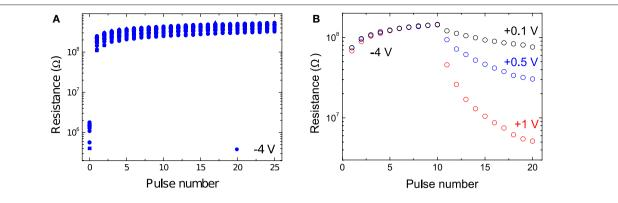
**FIGURE 4** | **(A)** Device response to the application of multiple RESET pulses of -4 V. **Supplementary Figure 1** shows the results for varying RESET amplitudes. **(B)** Device response to the application of multiple SET pulses of varying amplitudes of +0.1 V (black), +0.5 V (blue), and +1 V (red). 10 RESET pulses of -4 V are applied to increase the resistance before the application of the potentiation pulses.
