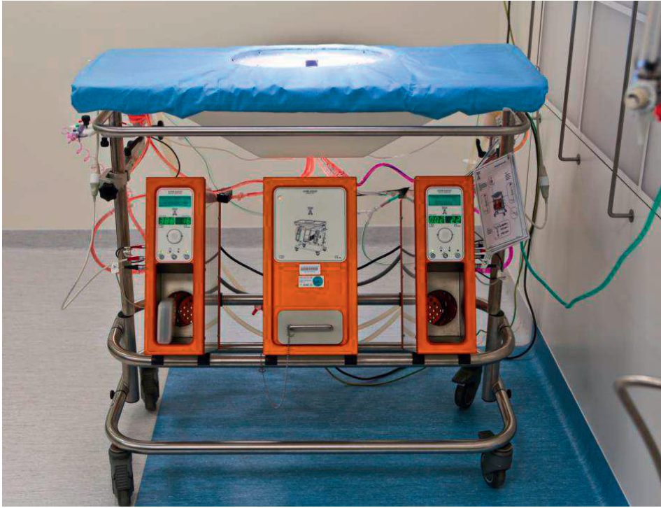
Figure 5. Photo of the Liver Assist, a perfusion device for preservation of human donor liver developed by researchers in Groningen (Organ Assist, Groningen, the Netherlands). The Liver Assist is a pressure-controlled system that allows perfusion of a donor liver via both the portal vein and hepatic artery. The temperature range can be adjusted between 10 and 37 °C.
