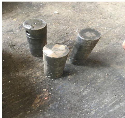
Gambar 15 shaft pinion gear rusak
