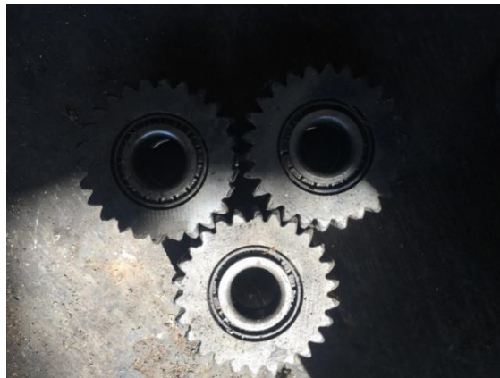
Gambar 13 toth pinion gear rusak
