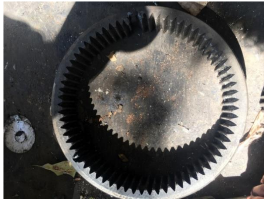
Gambar 12 ring gear rusak
