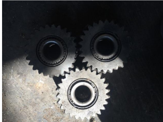
Gambar 14 bearing pinion gear rusak
