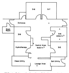
FIG. 1. Schematic drawing of the burn unit showing patient rooms and contiguous areas. The Xs indicate air sampling sites.
