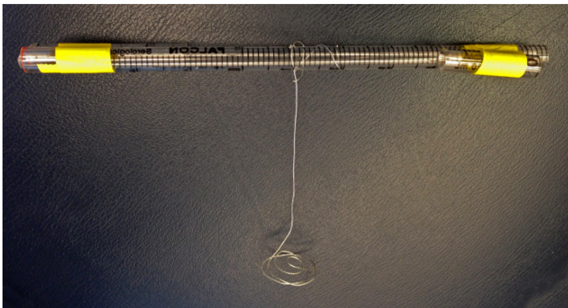
Figure 5: Lab made support for keeping lungs completely underwater. Device constructed from plastic pipettes and metal wire.
