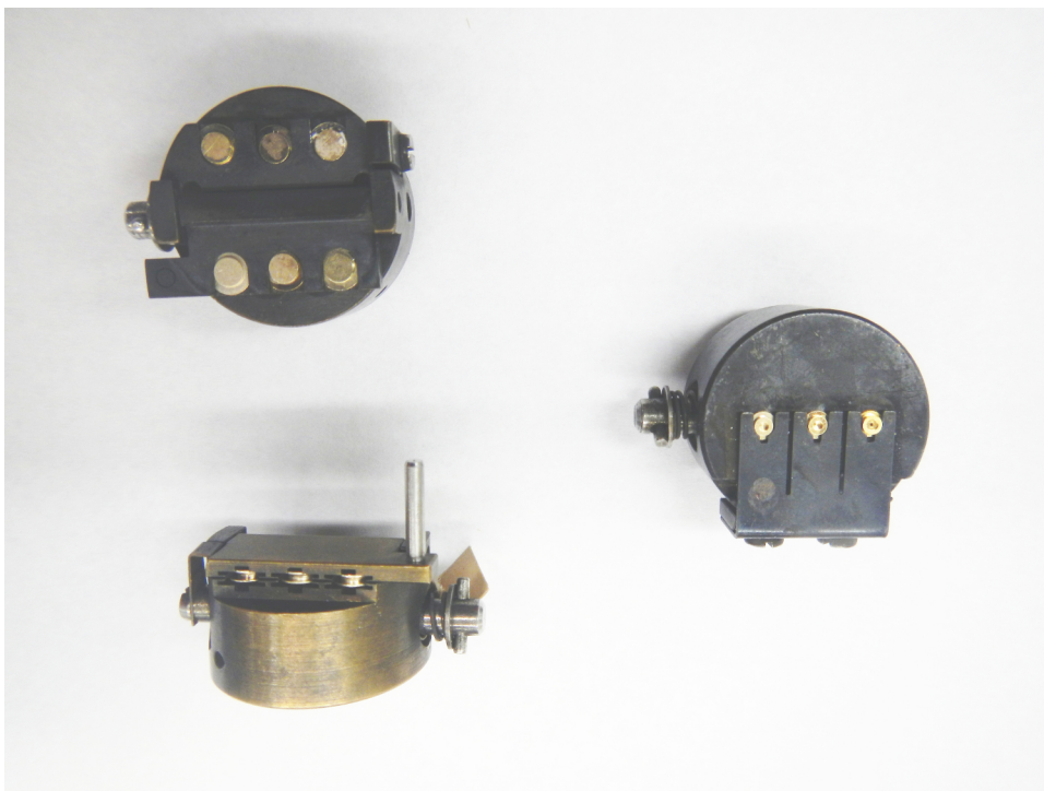
Figure 4. Two types of specimen mounts for freeze-fracture/etch procedures. (Left) A double replica specimen holder booklet is used for conventional freeze-fracture procedures performed without etching. The specimen is sandwiched between two gold specimen stubs and positioned in the brass booklet. The specimen is fractured by opening the booklet under vacuum in the specimen chamber (See freeze-fracture_movie1.mov). (Right) A mount used primarily for freeze-etching. The specimen is positioned on the gold stubs and locked into the brass holder. The specimen is fractured by gentle shaving with a razor blade fixed in the microtome arm. This configuration is preferred for etching procedures (See freeze-etch_movie2.mov).
