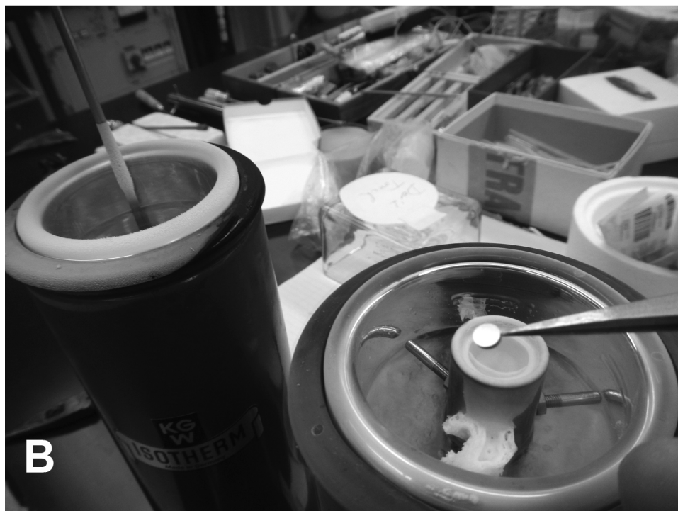
Figure 5. Preparation of a freeze-fracture specimen mount. The specimen is sandwiched between two gold mounts (A) and frozen in a well containing liquid nitrogen cooled propane (foreground) with subsequent transfer to a holding Dewar containing liquid nitrogen (background) (B).
