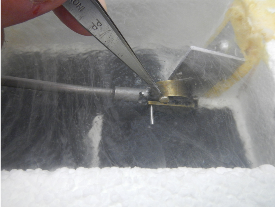
Figure 6. Demonstration of positioning of a frozen freeze-fracture specimen into the double replica specimen holder booklet in preparation for introduction to the specimen chamber of the freeze-fracture/etch plant.
