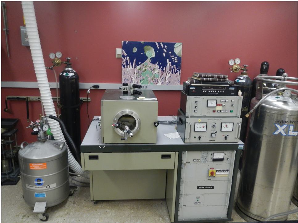
Figure 1. Layout of a commercial freeze-fracture/etch plant. At far left is a pressurized Dewar feeding cooling liquid nitrogen to the specimen stage and cooling microtome arm under controlled conditions. At center is the unit with specimen chamber and electronic control panels to the right. At right is an additional liquid nitrogen tank on which the vent gas is used to bring the specimen chamber to atmosphere.
