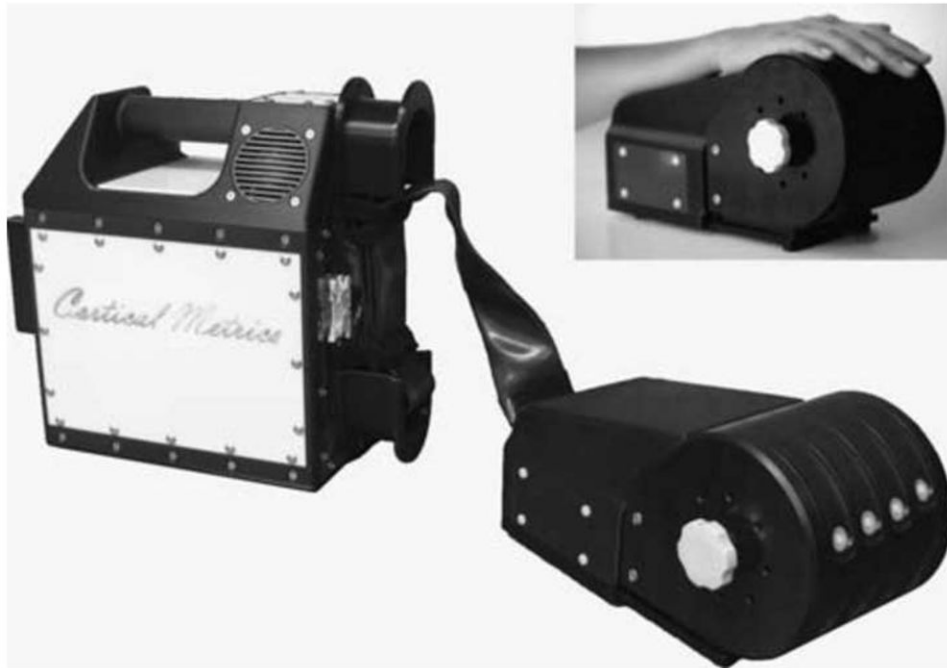
Figure 1. Four Site Vibrotactile Stimulator. Each of the four probe tips is positioned by rotating the four independently-positioned drums to maximize contact between finger pads and the stimulator tips. During an experimental session, subjects were seated comfortably in a chair with their arm resting on the arm rest attached to the head unit of the device. Digits D2 through D5 were then positioned for vibrotactile stimulation.
