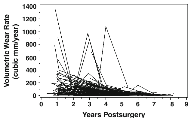
Fig. 2 A spaghetti plot of the estimated volumetric wear rates with time for the entire cohort ( n = 102 hips) is shown. Each line represents one hip. The variation in the estimated volumetric wear rates decreases with time as more data points became available for inclusion in the analysis.
