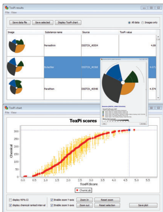
Fig. 1. Example of relationship between Results and Chart windows. The upper panel shows sorted ToxPi results, with the highlighted reference chemical (rank #2) signified by the bold square and cross-hairs on the lower panel. Inset : pop-up high-resolution window showing individual chemical's ToxPi and information
