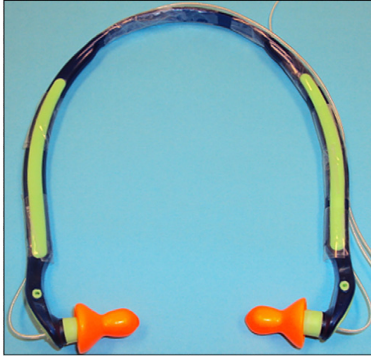
Fig 4. Sensors were attached to a commercially available band-type hearing protector. A hole was made in each auricular part to fit 2 sensors, and the third was attached to the middle of the band.
