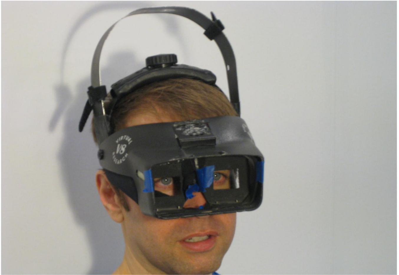
Fig. 2. The modified V8 HMD, with display elements removed so that subjects could see through the casing to the world-fixed display. The Hiball tracker not shown in this picture was mounted on the top loop during use.
