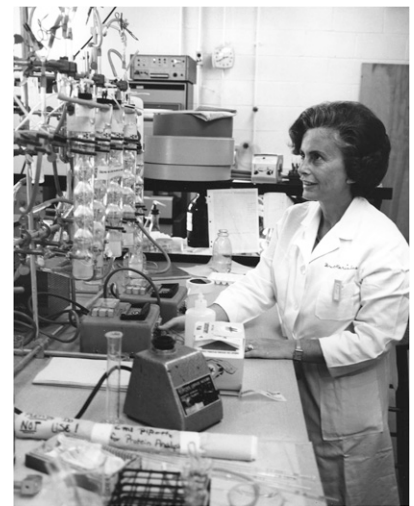
Maria Gordon Buse, MD, in front of a rack of Langendorff baths used to perfuse isolated beating rat hearts circa 1972. These studies resulted in important findings about cardiac fuel metabolism and changes induced by epinephrine, glucagon, and nutritional states with continuing relevance to diabetes treatments today (courtesy of the Waring Historical Library, MUSC, Charleston, SC).
