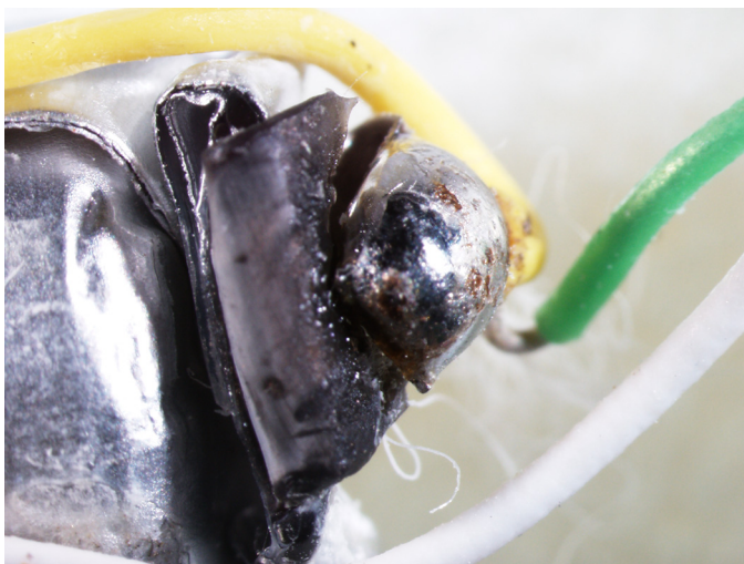
Fig. 8. A tin solder connection on a battery of an e-cigarette appears to have undergone some corrosion.
