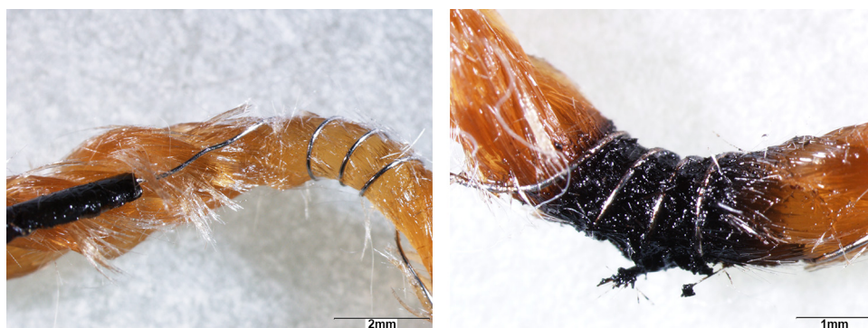
Fig. 5. Light microscope image of the nichrome heating element coiled around the vitreous fiber wick of an e-cigarette before ( left ) and after ( right ) use. Note the evidence of thermally decomposed organic substances and fragmented vitreous fibers in the vicinity of the heating element.
