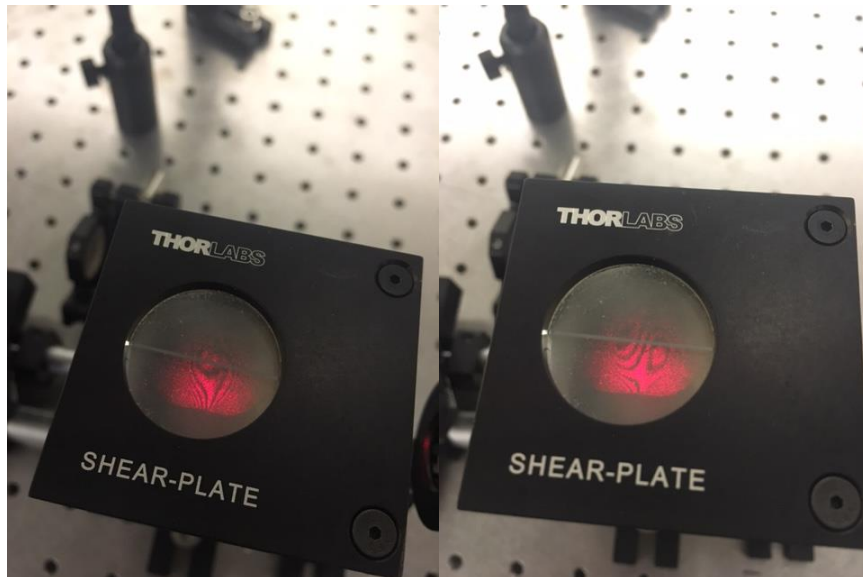
Not Collimated (with spherical aberrations) Close to collimated (with spherical aberrations)
