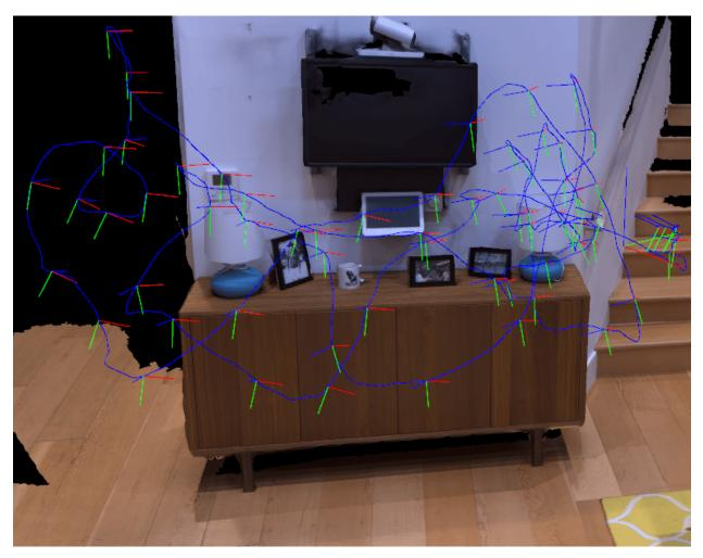
Figure 4.3: This figure shows the training scene used for all our indoor scene reconstruction experiments. We used about 200 real stereo images in real-scene training experiment, these views are shown in this figure by 3D axis along with the camera trajectory visualized by the blue curve. The 3D reconstruction was built using the method described in (Whelan et al., 2018).
