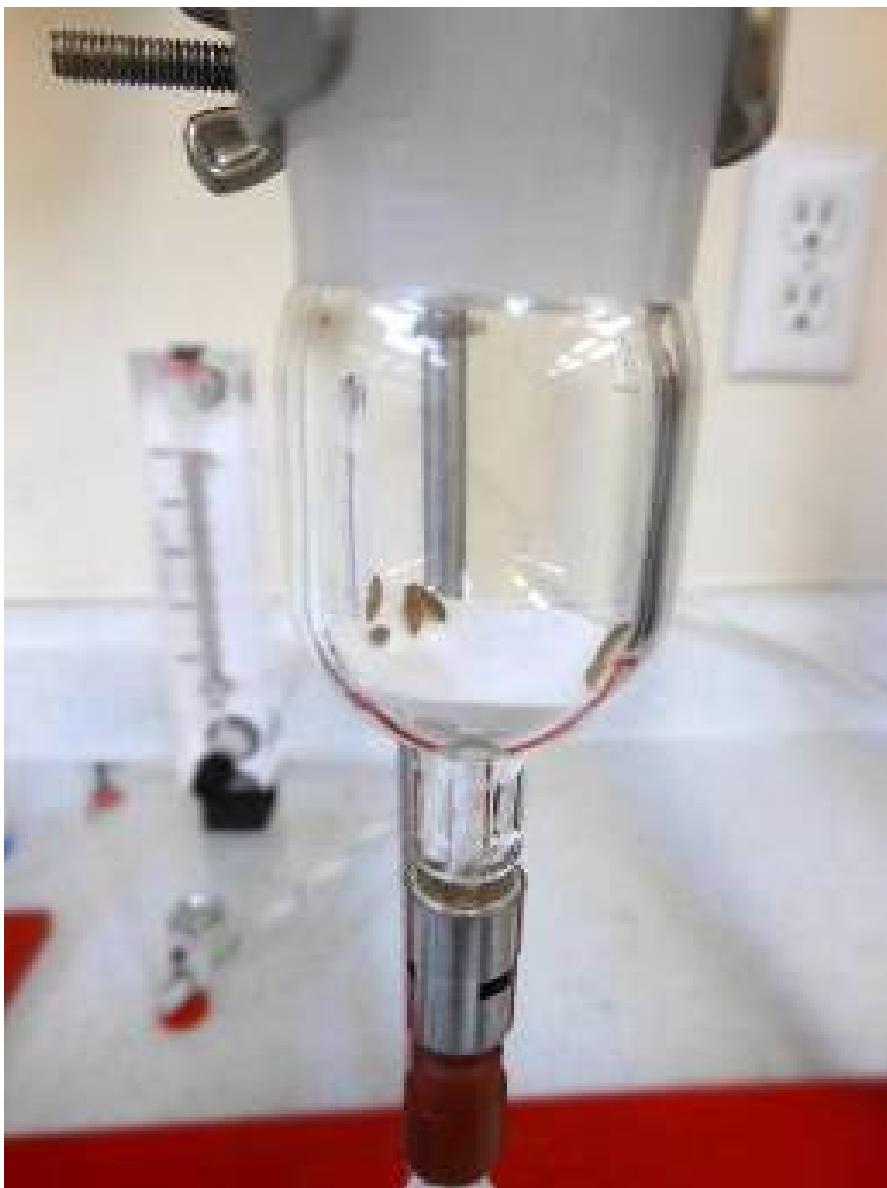
Figure 4: Multiple adult virgin female Thylodrias contractus placed together to collect potential sex pheromone in the head space above with the Porapak Q column.
